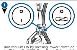
Turn vacuum ON by pressing Power Switch on (I - ON and O - OFF). Press Brush Roll switch to run the PowerBrush for carpet cleaning (Brush Roll is ON when light on switch is illuminated). See page 15 to maintain the Brush Roll.
