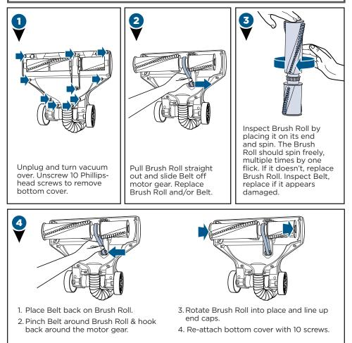
**NOTE:** If an object becomes lodged in foot and brush shuts off, turn vacuum OFF and unplug from electrical outlet. Remove obstruction and brush will automatically reset when vacuum is plugged and turned back ON.
