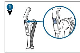
Locate the Suction Control setting on the vacuum handle. Adjust Suction Control for plush carpet or low carpet for easy multi-surface cleaning.
