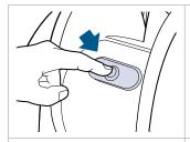
1. Turn Power Switch to OFF position. Unplug power cable from outlet.
