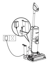
To charge the appliance, place the appliance on the charging base and plug the adaptor into a power outlet.
