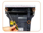
1. Undo the below three screws. The roller brush and the belt can be removed for replacement.
